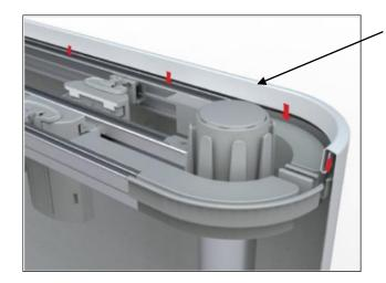
Beginning on one end, insert the leading edge of the print into the top graphic rail and continue feeding it in along the rail until the entire top edge of the print is loaded. Repeat the process along the bottom rail until both top and bottom edges of the print are loaded into the Graphic Rails.
