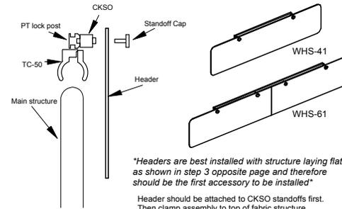
*"Headers are best installed with structure laying flat as shown in step 3 opposite page and therefore should be the first accessory to be installed"*
