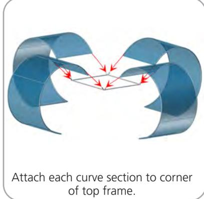
Attach each curve section to corner of top frame.
