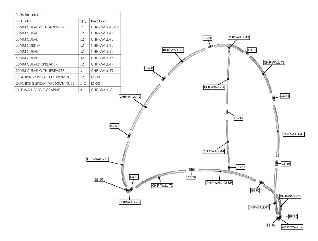
**CHIP-WALL FRAME ASSEMBLY:** Assemble unit by laying tubes flat on the floor. Connect the tube rails following the labels by matching number to number.
